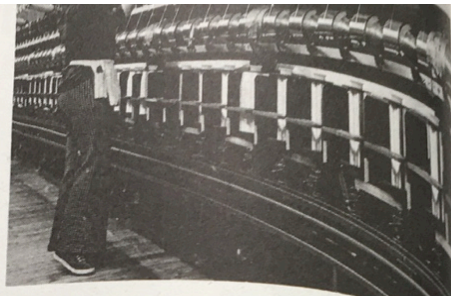
17.2 Spinning filament yarns. As filaments are formed, they are combined, formed into yarns, and wound onto bobbins at the base of the machine. Completed bobbins are placed at the top, then collected for transport to other areas. Empty bobbins are left to be exchanged with a full bobbin. (Celanese Corporation)
